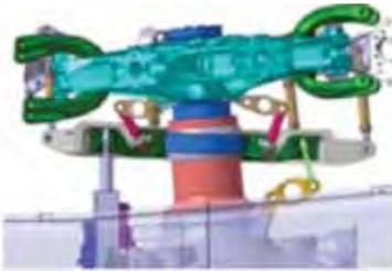
Figure 6 MR Assembly – (Swashplate, Pitch Control Rods, Scissors)
