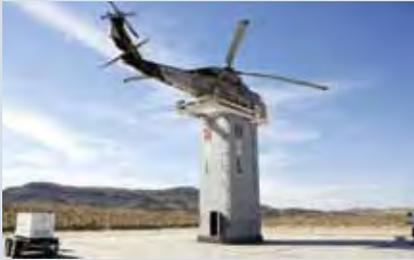
**Figure 2** Helicopter Hover Fixture at HFI Facility
