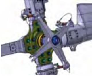
Figure 5 Tail Rotor System
