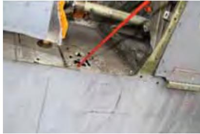
**Figure 17** Trailing Edge Spar Damage for Shot 6
