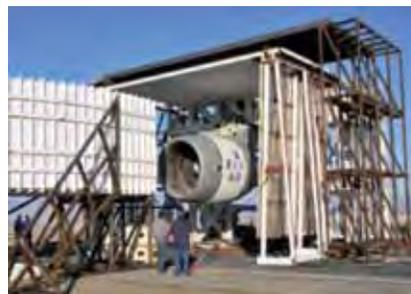
**Figure 8** Large turbofan engine hanging on its test fixture prior to MANPADS testing. Note the size of engine and test fixture compared to the two people in front of the engine. Note the size of engine and test fixture compared to the two people in front of the engine. (US Navy Photo)
