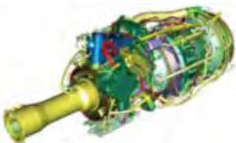
Figure 8 GE38-1B Turboshaft Engine
