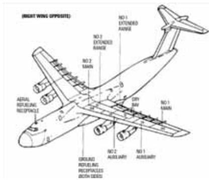
**Figure 1** Wing Integral Fuel Tanks
