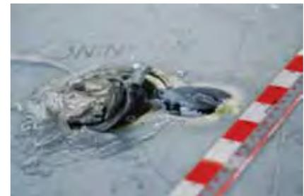
**Figure 13** Typical Upper Surface from Ballistic Test, Event 3
