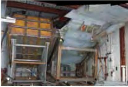
**Figure 7** Surrogate Right Hand Wing with Water Reservoir
