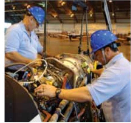
**Figure 9** Engine maintenance specialists position an upgraded PT6A-68 turboprop engine in a T-6 Texan II aircraft at Randolph Air Force Base, Texas. (US Air Force photo by Steve Thuro/Released) 091214-F-SS509-001
