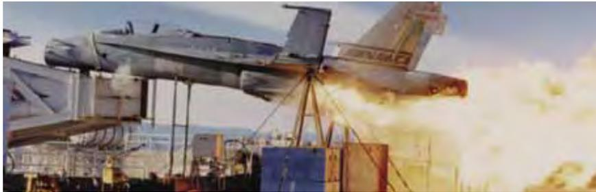
**Figure 6** F/A-18 Fuel System Joint Live Fire Testing
