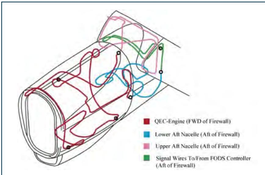
**Figure 6** C-130J Engine Nacelle Fire Detection Loops
