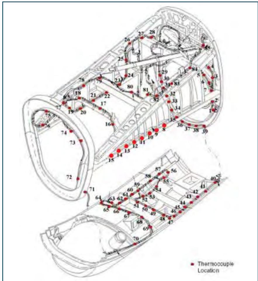
**Figure 7** Thermocouple Locations Placed Along Fire Detection Loop
