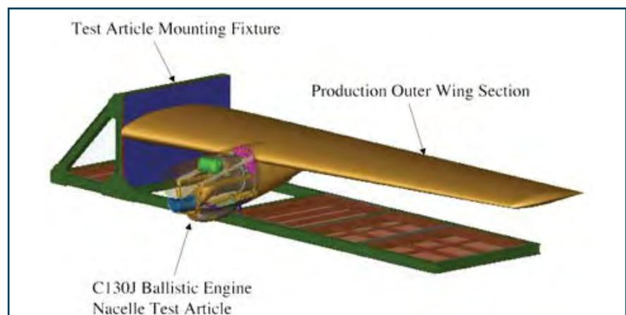
Figure 9 C-130 ENFEE Test Article Fixture: Schematic
