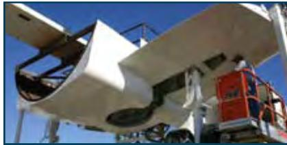
**Figure 2** P-8A Main Landing Gear Bay “Iron Bird” Simulator
