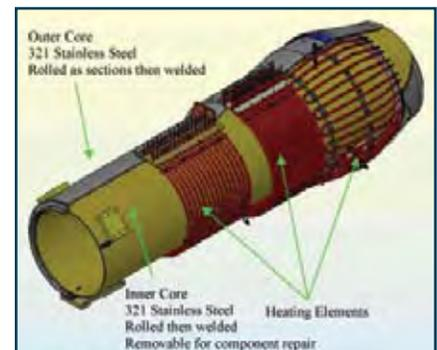
Figure 2a Replica Engine Core with Heaters Installed
