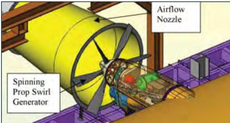
**Figure 10** Engine Nacelle with Spinning Prop Swirl Generator
