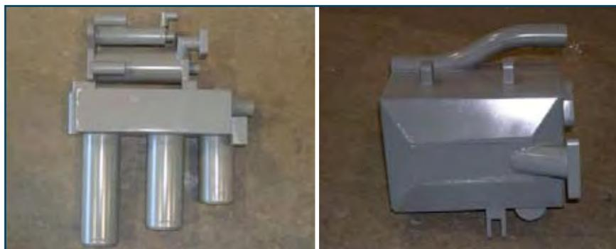
**Figure 5** Replica Oil Filter (Left) and Replica FCOC (Right)
