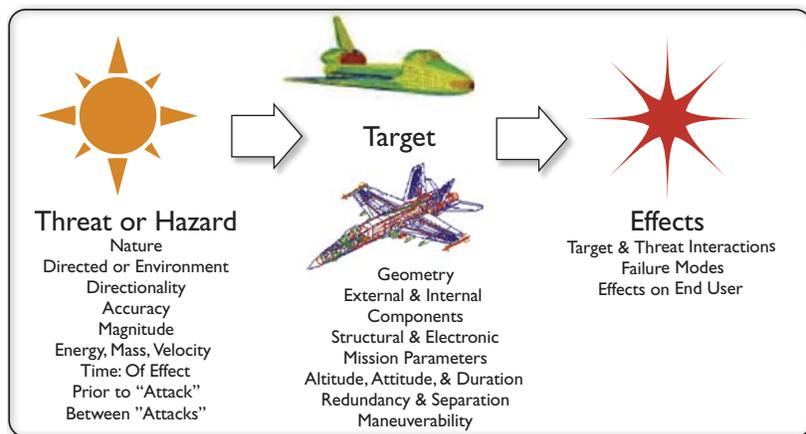
Figure 5. Model considerations for computing space shuttle and combat aircraft vulnerabilities?
