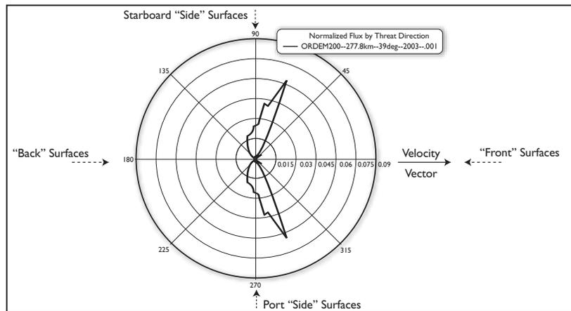
Figure 4. Directionality of the NASA orbital debris environment perpendicular to the orbital plane for spacecraft in low-earth orbit as viewed from Zenith?
