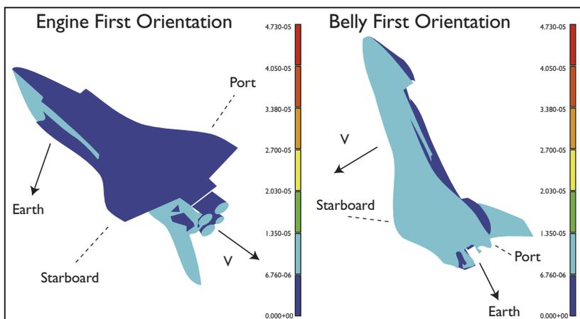
Figure 3. BUMPER graphical output showing probability of impact by meteoroids for two shuttle flight orientations<sup>2</sup>
