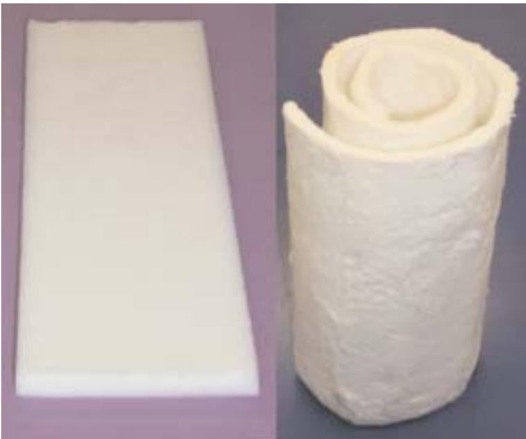
Figure 3. Aerogel board (left) and flexible aerogel blanket (right).
