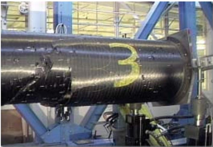
Figure 2.. Ultimate-to-failure Static Test
