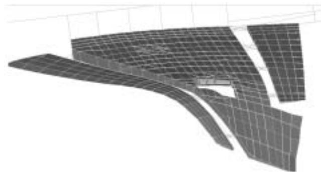
Figure 10. Sample Case 3. Typical Wing Tip Damage – Mach = 0.95
