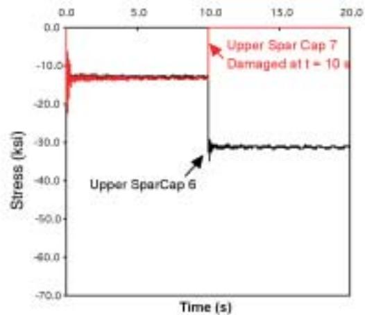
Figure 5. Spar Cap Stresses Before and After Damage
